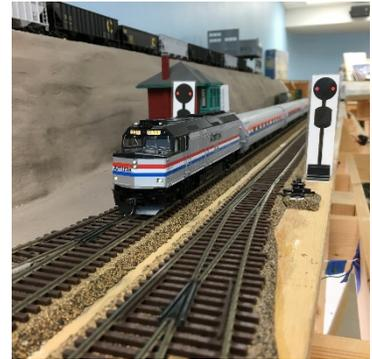
Layout control: NCE DCC provides layout control. A central dispatcher directs operations through JMRI block detection and remote turnout control.
