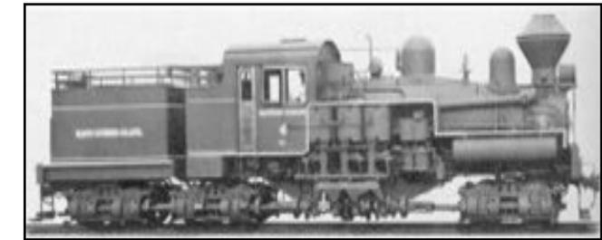
in the drive trucks ability to slide under high torque. This caused Shays to run off the rails when going around rail/track curvature. The problem is not noticeable on straight runs, but becomes apparent around curves. Shays were built in 4 major classes: The Class A with 2 cylinders and 2
